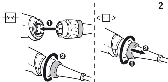
Connecting and detaching the mains power cable - see Fig. 2.
