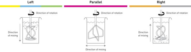
For low-viscosity mixtures (e.g. paints and emulsions). Works from top to bottom – this means the material is transported downwards. Prevents material splashing. Thorough mixing of the material for flowing mixtures. Prevents air pockets, for example in levelling compounds and fillers. For high-viscosity, compact mixtures. Acts like a screw in the mixture and transports the material from bottom to top.
