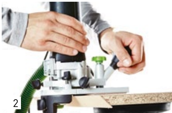
2 Then mill the workpiece flush.
